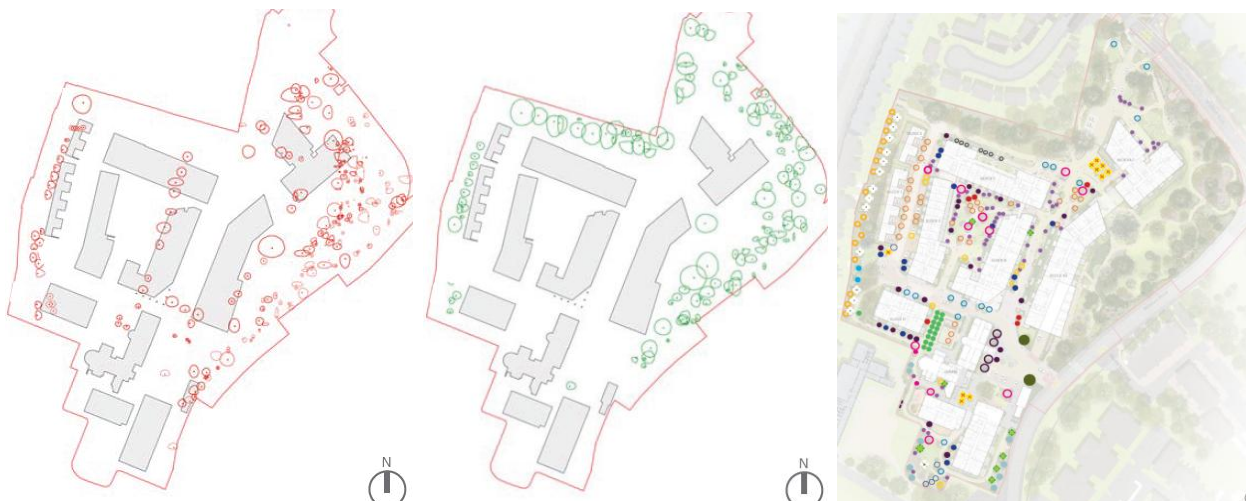
Figure 9.13: (a) Trees to be removed, (b) trees to be retained, and (c) proposed trees
